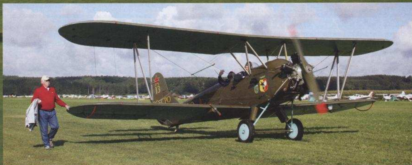
Above: From Wiener Neustadt in Austria came this Polikarpov PO.2 (OE-CPO), which in reality is a CSS-13, which now has a 125hp Shvetsov M-11D 5 cylinder radial engine. (Photo, Geoff Jones)
